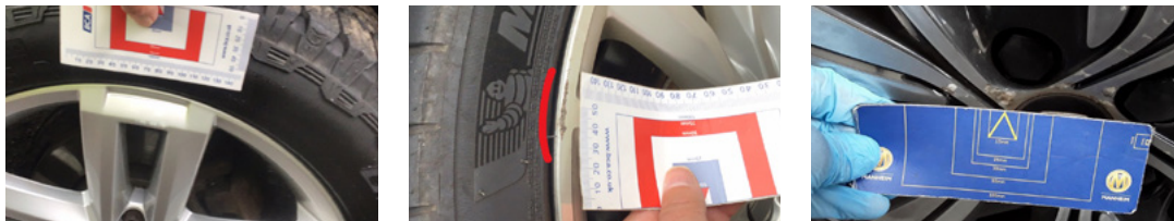
CHARGES APPLICABLE TO OVER 50MM. IMAGE 2 SHOWS 40MM WHICH IS WITHIN TOLERANCE.
